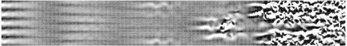
FIG. 1: Contour plot of streamwise velocity fluctuations in a plane parallel to the wall in the core of the boundary layer during bypass transition induced by free-stream turbulence. The flow is from left to right. DNS simulation by ? .
