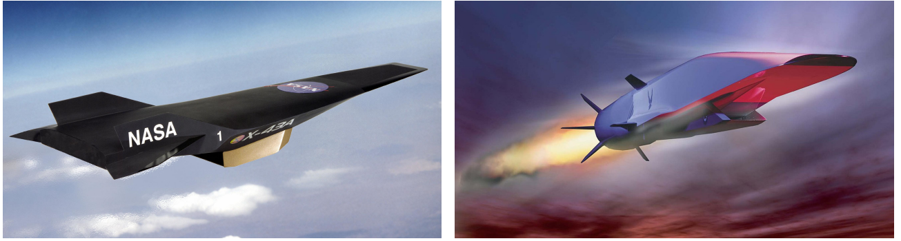
Fig. 19 Hypersonic airbreathing vehicles. Left: X-43A (image from https://www.nasa.gov/ ). Right: X-51A (image from https://media.defense.gov/ ).
